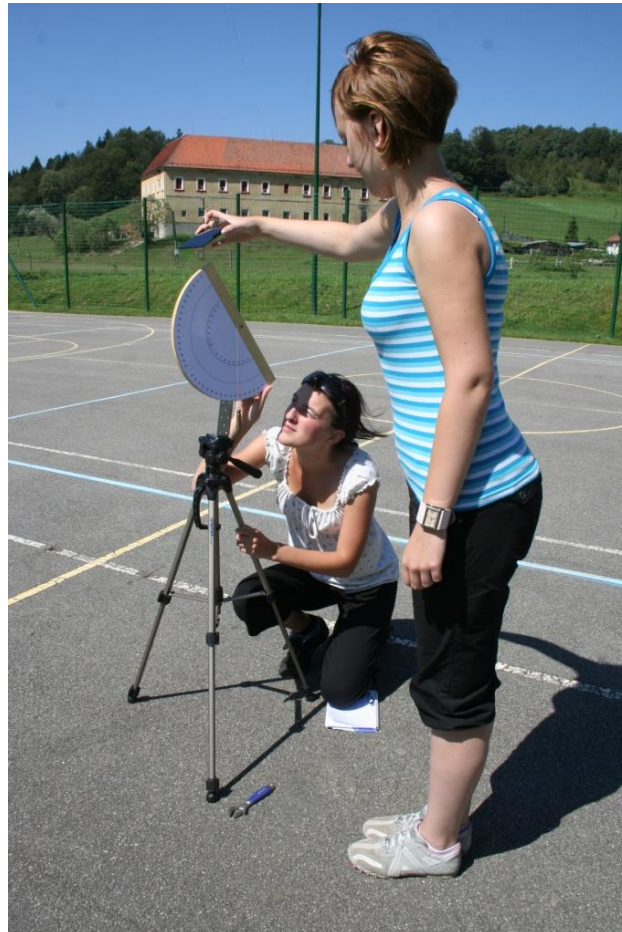
Figure 1: Measurement of the height of the Sun with inclinometer.
